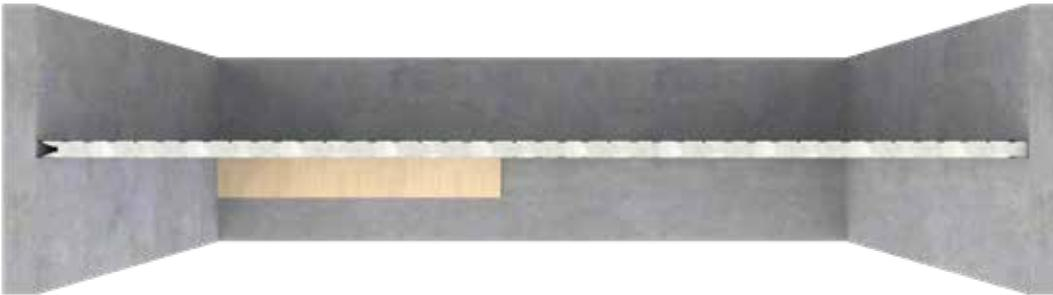
Once the last panel is positioned in between the two angled panels, push the panels into the track to snap each panel into place.
