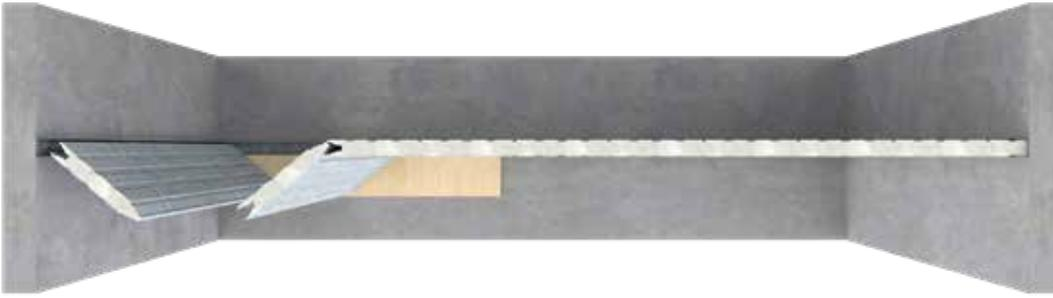
Wedge two panels into the C-track, make sure that one panel is placed within the track and the other panel is placed within the already installed panel.
