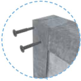
The corner fixings are to be screwed in on a 45° angle. There must always be 2 fixings at every corner.
