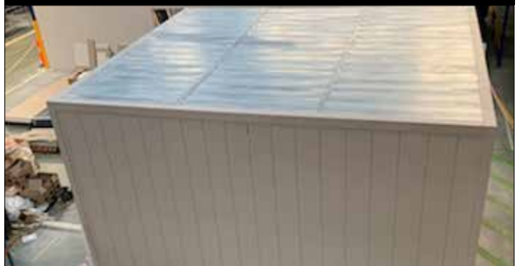
K8 SUPAPANEL® verberation chamber - Acoustic testing
